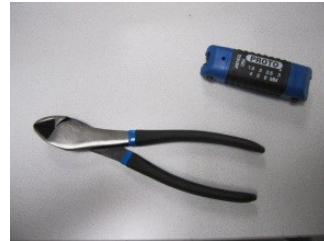
(20) Part Number # 069-67-123 One Heavy Duty Diag Side Cutters (21) Part Number # J4974CG One Fold Hex Key 1.5mm – 6.0mm Allen
