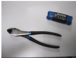
PN # J4974CG One Fold Hex Key 1.5mm – 6.0mm Allen PN # 069-67-123 One Heavy Duty Side Cutters
