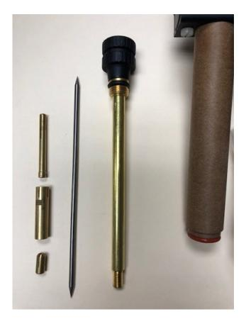
Be sure red ring is on end of torch and finish with insulator and gas lens
