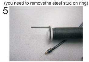
Install the Nozzle Insulator and the Gas Lens on the torch.
