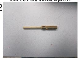
Identify the Electrode Collet and insert it into the case.
