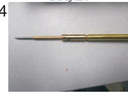
Install the ring insulator and the ring onto the torch shaft.
