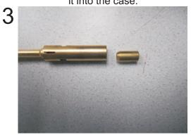
Insert the Tungsten into the Electrode Case, adjust stickout and tighten.
