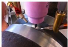
TiP TiG Orbital Tractor is a rugged, light weight precision TiG weld head for use with the TiP TiG HotWire Welding Process, suitable for all pipe sizes from 4" (100 mm) pipe up to an unlimited size, including flat plate.
